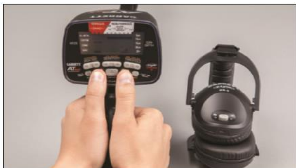
PAIRING: Switch on headphones and hold within 0.6 meters (2 feet) of AT Max, then press and release Z-Lynk buttons (IRON AUDIO and FREQ) simultaneously.
